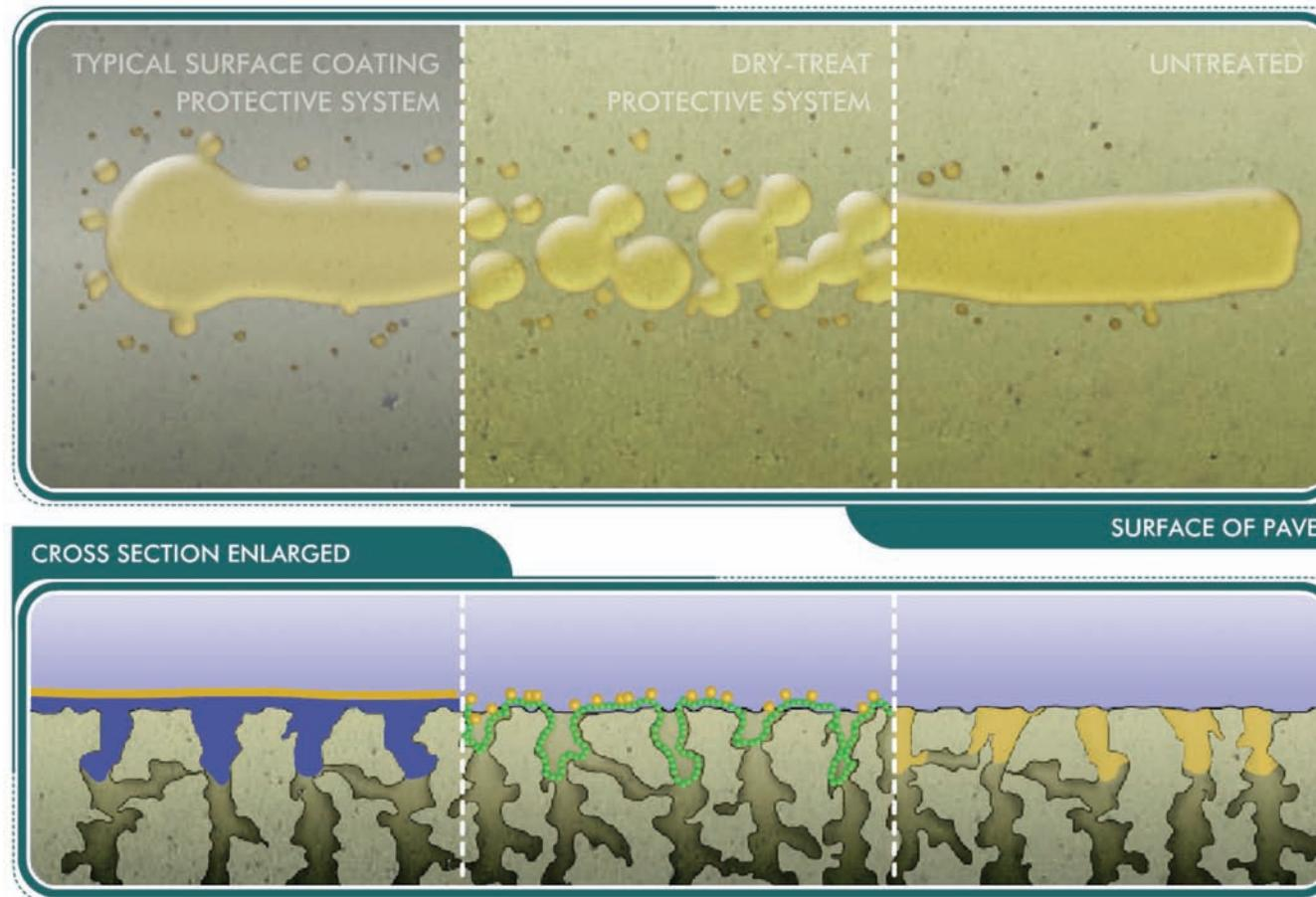
Dry-Treat sealers alter the surface energy of the treated material to a level below that of liquids, preventing their entry and thus staining. All Dry-Treat sealers are impregnating, and penetrate deep into the surface of the treated material. This deep penetration is critical to giving extreme longevity and protection against weathering and traffic which could remove the treatment.
